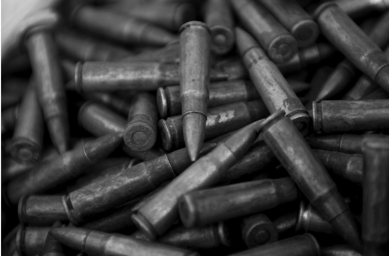
Figure 3.10 (See color insert.) Ammunition under investigation in Baghdad, Iraq, in 2006. Closer inspection of the casing head stamp reveals ППZY for Prvi Partizan; the year 2002 is also marked. Other identifying characteristics to look at include the brass casing and the distinctively red primer sealant, a color unique to Prvi Partizan. (U.S. Air Force image; photograph by Technical Sgt. Adrian Cadiz.)
